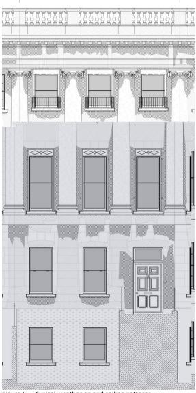
Figure 6 Typical weathering and soiling patterns
